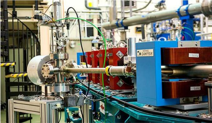
The Science & Technology Facilities Council (STFC) is coordinating production of the cavities through Daresbury, where it will perform acceptance testing, including radio frequency (RF) tests in cryogenic conditions. They will be also responsible for ensuring that the cavities are literally spotless before they are locked away inside cryogenic tanks at France's CEA Saclay laboratory and delivered for installation in Lund.
