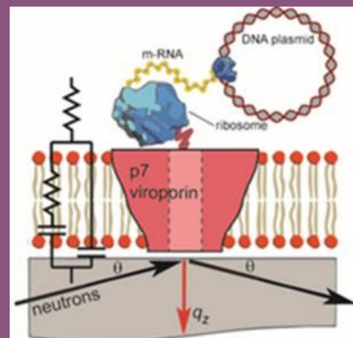
The cell-free preparation of supported bilayers containing p7 and NR and EIS measurements (not to scale). For neutron reflectivity, membranes were formed on quartz and an incident neutron beam was transmitted through the substrate and reflected from.
